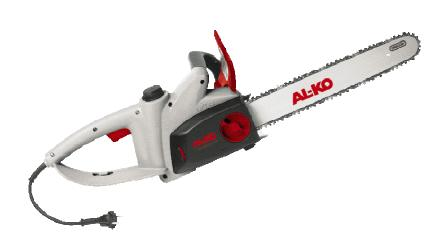
The ergonomics of this model make its ideal for domestic use by allowing fatigue free working in all positions, while safety is maximised by the fast acting 0.1 second chain brake. The KE2200/40 features a powerful 2200 watt motor with a 40cm guide bar, running Oregon 3/8" chain with automatic oiling. This model also benefits from a tool free chain tensioner for rapid adjustments in the field.
